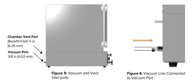
Use clamps to secure tubing to the Vacuum Port and Chamber Vent Port (backfill inlet).
